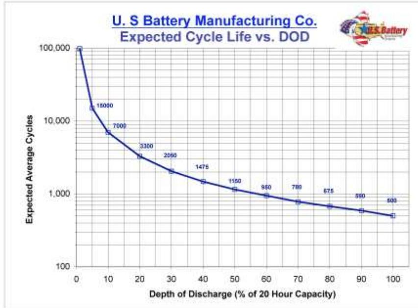
**Figure 2: Discharge Depth vs. Battery Life**
