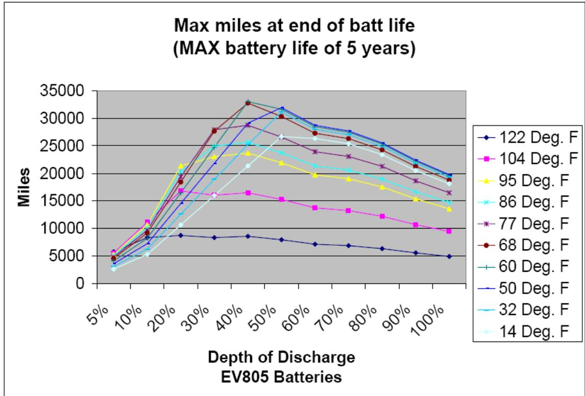
Figure 6: AGM 230 AH Batteries Max Miles vs. DOD vs. Temp.
