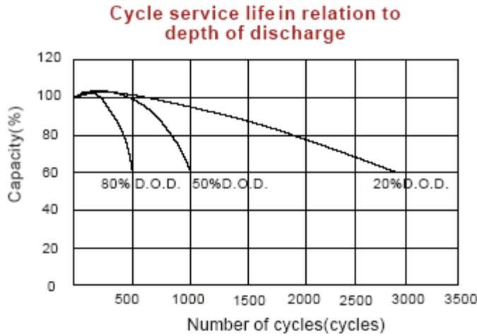
Figure 4: Discharge Depth vs. Battery Life
