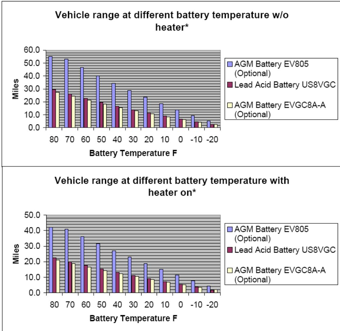
\*These tests were performed with an EXV2 model equipped with an enclosed cab. Vehicle weight with one driver was 2050 lbs. with the US8VGC & EVGC8A-A batteries, 2400 lbs with EV805 batteries. This vehicle was driven on a course that was a 3 mile loop. It has two complete stops and mostly flat but has some moderate hills.
