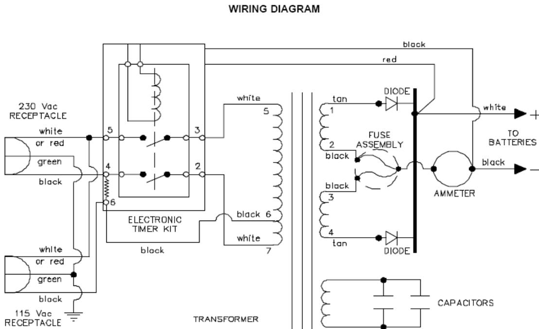
**Figure 11: Charger Wiring Schematic**
