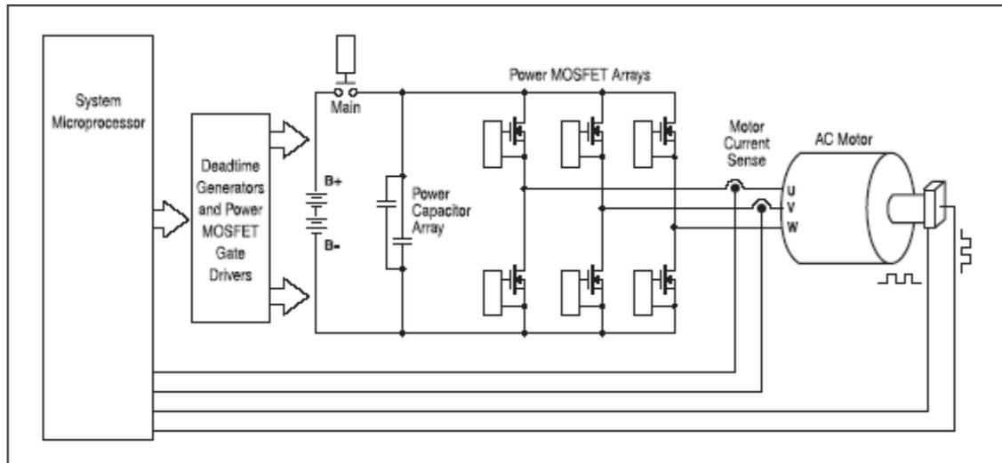
**Fig. A-2** *Power section topology.*
