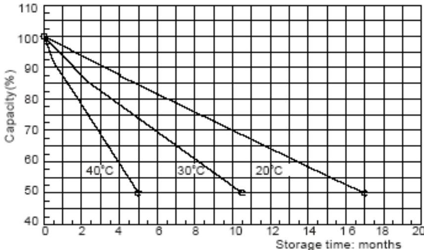
**Figure 7: AGM Batteries Self-discharge Characteristics**
