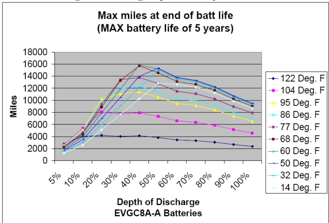
Figure 5: AGM 180 AH Batteries Max Miles vs. DOD vs. Temp.
