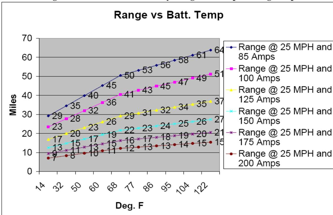
**Figure 9: AGM 230 AH Battery Range vs. Temp. vs. Avg. Amp Draw**
