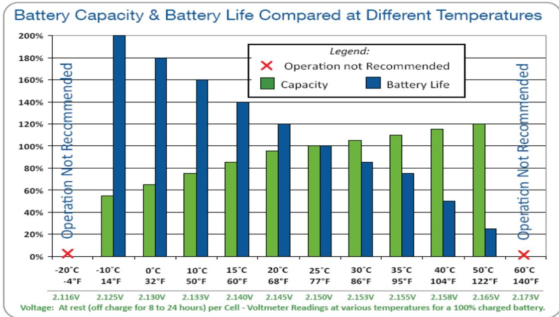
Data provided as representative only. Battery voltage, capacity and life will vary with actual environmental conditions and operator driving habits. Operation above 50°C / 122°F and below -10°C / 14°F is not recommended.
