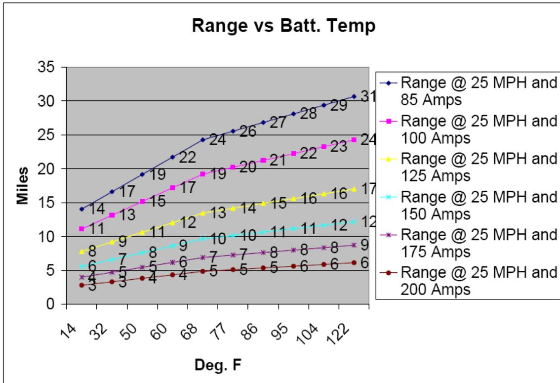
**Figure 8: AGM 180 AH Battery Range vs. Temp. vs. Avg. Amp Draw**
